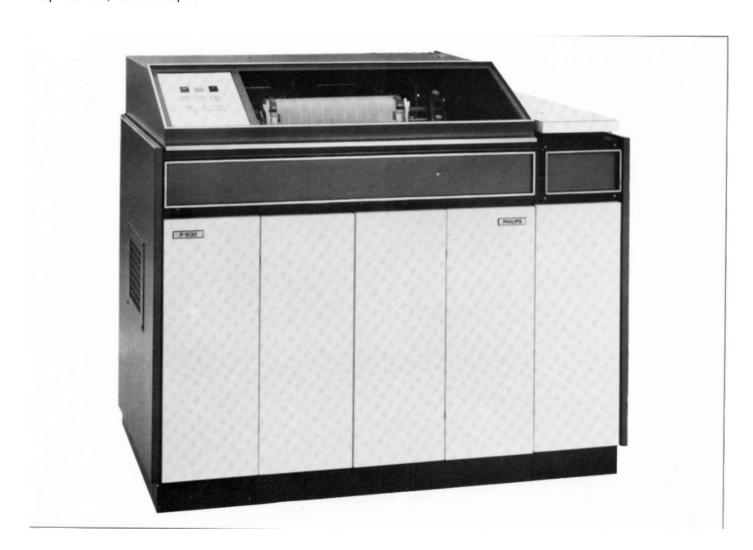
This device plots output from the P1000. Digital signals cause a plotting pen and a plotting drum to move in steps, thus drawing a graph. Two models are offered, giving plotting widths of 11 in (28cm) and 29.5in (75cm).
