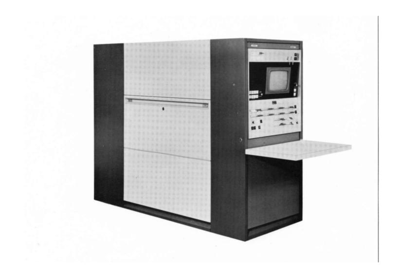
This machine is designed for use with the P350 Office Computers: as soon as an instruction 'Read' is reached in the program, the card reader switches on and follows the program. Half a minute after instructions stop flowing, the unit switches itself off to save running time.
