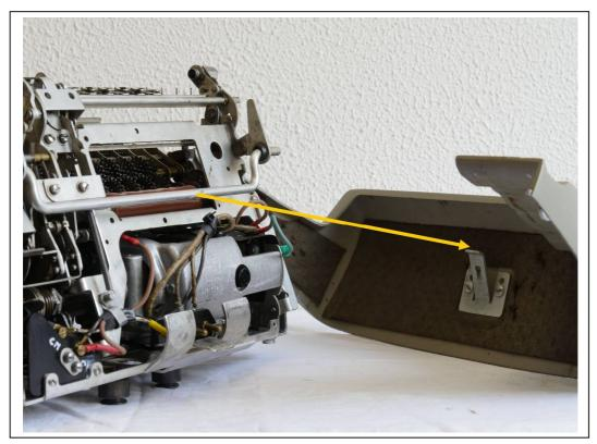
5. Finally four bolts (here white plastic) prevent that the machine can move inside its casing. This way the entire closing mechanism is secured.
