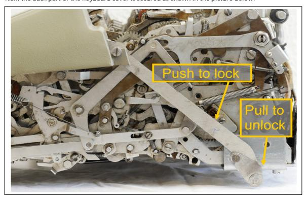
4. The next step is to mount and secure the back part of the casing. Tighten the feet which were loosened in step 1.
