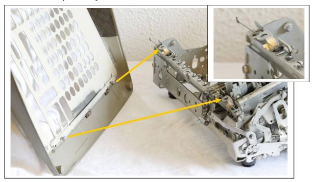
3. Next the back part of the keyboard cover is secured as shown in the picture below.
