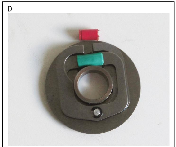
Picture C shows the assembly. In picture D it is mounted in the mechanism. Now there is no play while still there is flexibility in the mount.
